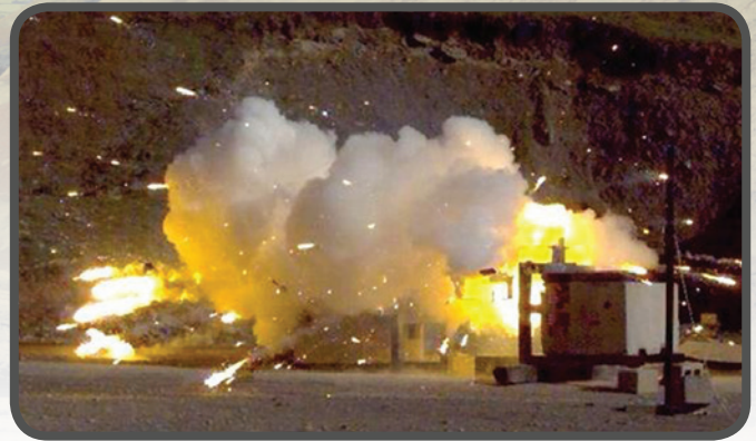
STANAG 4241: Bullet Impact Test.
