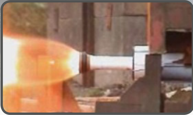
Functioning of a rocket motor as part of an end of life analysis study.
